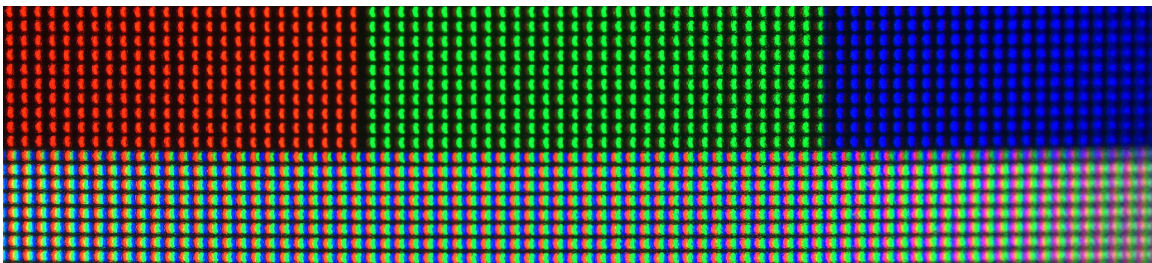
ACTUAL PHOTO OF LCD SCREEN TAKEN WITH A MACRO LENS ADAPTER ON AN IPHONE
